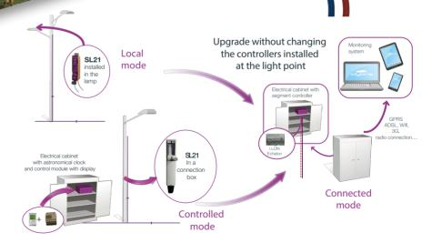
The SL21 uses **power line carrier** technology (via the existing power grid) and operates using the **LonWorks® protocol**, **which is open and interoperable** (non-proprietary).
